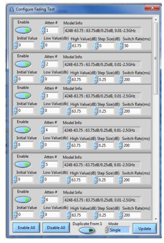
The system automatically determines the allowed limits for each parameter. Each attenuator has the following parameters:
