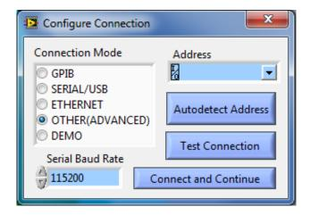
Autodetect will provide a list of controllers and their addresses. Select the desired controller and hit connect to continue.
