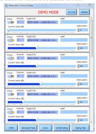
5. To save the connection information, text entered to label each channel, and attenuator state hit the save button on the bottom of the control center window, then select either a preset or a custom save file name.
