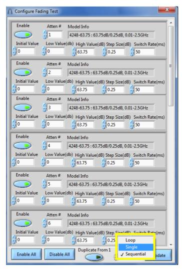
**Loop:** Continually loop through the selected test profile. The increment is reversed each time an attenuator hits its limit.
