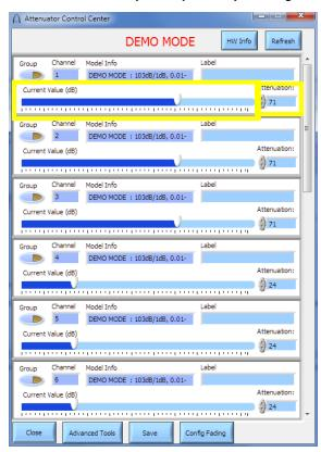
2. Selecting "Group" allows the user to control multiple attenuators to be controlled at once
